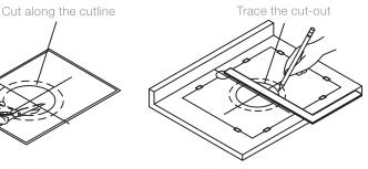
• Drill pilot hole inside the perimeter line of the template.
