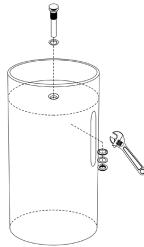
4. Screw a flanged tail piece to the pop-up drain inside the cavity of the basin. Access is provided through the waste opening on the back of the basin. Flanged tail-piece should be tall enough so that it is accessible through the waste opening on the back of the basin.
