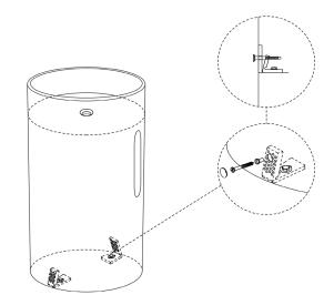
9. Apply a thick bead of adhesive silicone caulkling to the base of basin where it meets the floor.
