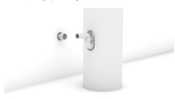
6. Rotate the basin so the back is facing towards the finish wall.
