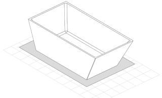
7. Create an opening in the finished floor with ample space to accomodate a P-trap assembly or flex-hose assembly.
