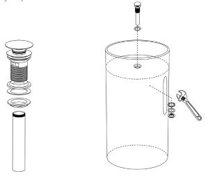
4. Screw a flanged tail piece to the pop-up drain inside the cavity of the basin. Access is provided through the waste opening on the back of the basin. Flanged tail-piece should be tall enough so that it is accessible through the waste opening on the back of the basin.
