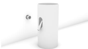
4. Connect a P-Trap to the flanged tail piece so that it produces out of and past the inner cavity of the basin.
