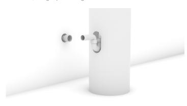
6. Rotate the basin so the back is facing towards the finish wall. Lift the basin and then lower it down into position using your outline (from step 1.) as a reference.
