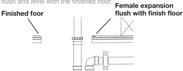
Once in place and flush with the finished floor – secure the female expansion joint and P-trap to a floor joist with a steel-strap to hold it in place.
