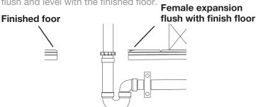
Once in place and flush with the finished floor – secure the female expansion joint and P-trap to a floor joist with a steel-strap to hold it in place.
