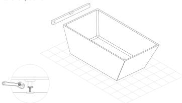
\*\*IMPORTANT\*\* - Water will only drain properly to the waste outlet if the bathtub is level.
