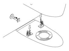
4. Turn toilet on its side (please protect the ground surface with soft material to prevent damage to toilet), and press new wax seal firmly around waste flange. apply a small bead of silicone sealant around toilet base.
