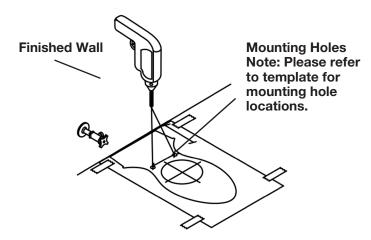
\*\***NOTE**: For floors less than 1-1/2" (38 mm) thick use a 5/32" bit. For floor thicker than 1-1/2" (38 mm) use a 3/8" bit for anchor (required) installation.\*\*
