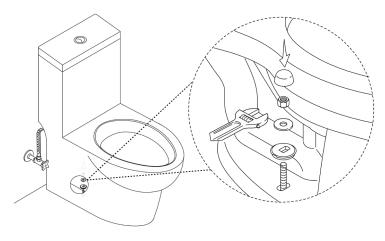
\*\*NOTE: Do not overtighten nuts. Porcelain is fragile and could possibly crack if nuts are overtightened.\*\*
