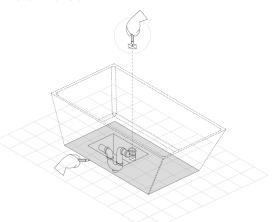
4. With the tub still in place mark the location and center-point of the drain outlet.
