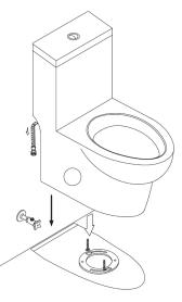
5. Press toilet down firmly on wax ring and flange until toilet is securely seated on floor.
