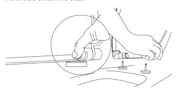
To re-install the seat. Align seat pins with the seat hinge sockets and apply downward pressure until you feel and hear a "click". This "click" will signify the seat pin is locking into position.
