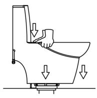
5. Place the bolt cap bases on the T-bolts and proceed to secure the toilet into place by fastening the washers and nuts to the bolt caps and T-bolts.
