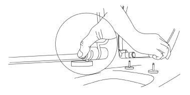
To re-install the seat. Align seat pins with the seat hinge sockets and apply downward pressure until you feel and hear a "click". This "click" will signify the seat pin is locking into position.
