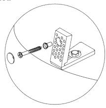
8. Tighten the toilet bowl mounting screws to the mounting brackets; place the finish caps on the heads.
