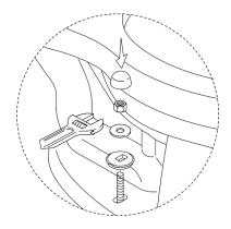
\*\*NOTE: Do not overtighten nuts. Porcelain is fragile and could possibly crack if nuts are overtightened.\*\*
