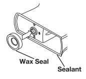
3. Install T-bolts in correct floor position and fasten closet flange.
