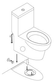
5. Press toilet down firmly on wax ring and flange until toilet is securely seated on floor.
