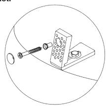
8. Tighten the toilet bowl mounting screws to the mounting brackets; place the finish caps on the heads.
