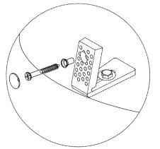
8. Tighten the toilet bowl mounting screws to the mounting brackets; place the finish caps on the heads.
