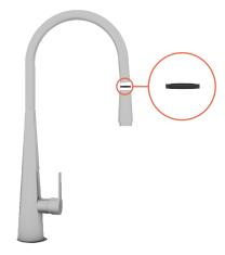
12. Test faucet and faucet head thoroughly. Make sure water flow is adequate. Inspect all aspects of faucet for leaks.
